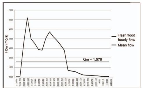
Figure 3. Hydrograph of the flash flood from 27th December 1995 to 2nd January 1996 at Gabru Hydrometric Station (Data source: ABA Jiu)
