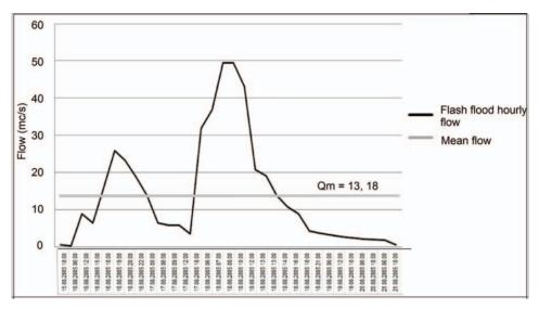
Figure 5. Hydrograph of the flash flood from 15th to 21th August 2005 at Dragoia Hydrometric Station (Data source: ABA Jiu)
