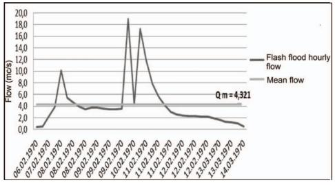
Figure 2. Hydrograph of the flash flood from 6th February to 14th March 1970 at Dragoia Hydrometric Station (Data source: ABA Jiu)
