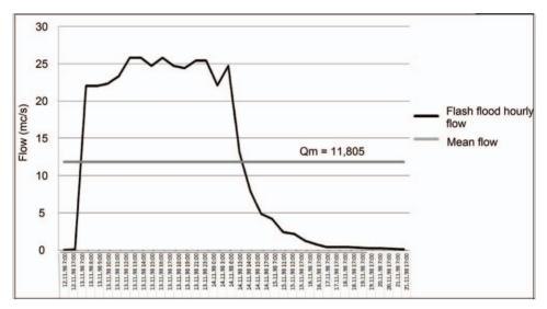
Figure 4. Hydrograph of the flash flood from 11th November 1998 to 19th November 1998 at Dragoia Hydrometric Station (Data source: ABA Jiu)
